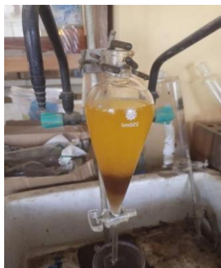
Plate I: Reaction set-up after the Transesterification
