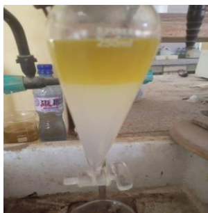
Plate II: Biodiesel being washed
