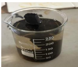
Fig 4: Fabricated biochar electrode immersed in KOH solution.
