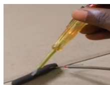
Fig 6: Electrical wire connection and conductivity testing of the fabricated biochar electrode.
