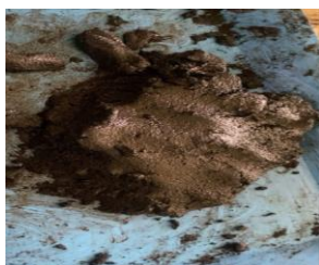
Fig 2: Biochar paste obtained for electrode fabrication.
