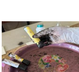
Fig 3: Fabricated paper mould and biochar paste formed into an electrode.
