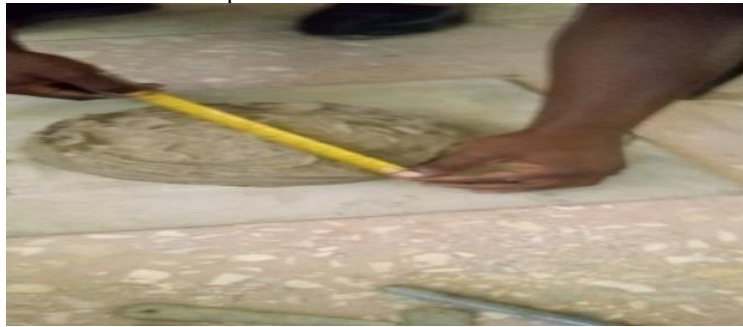
Figure 5: Spread Diameter Test of Foamed Concrete
