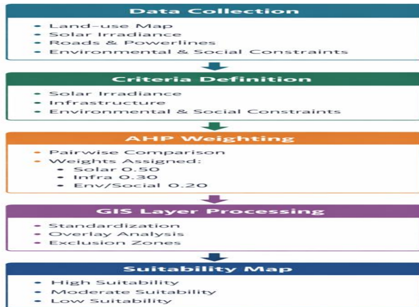
Figure 7a: GIS-based AHP Workflow for Solar Energy Suitability Assessment of Sokoto State
