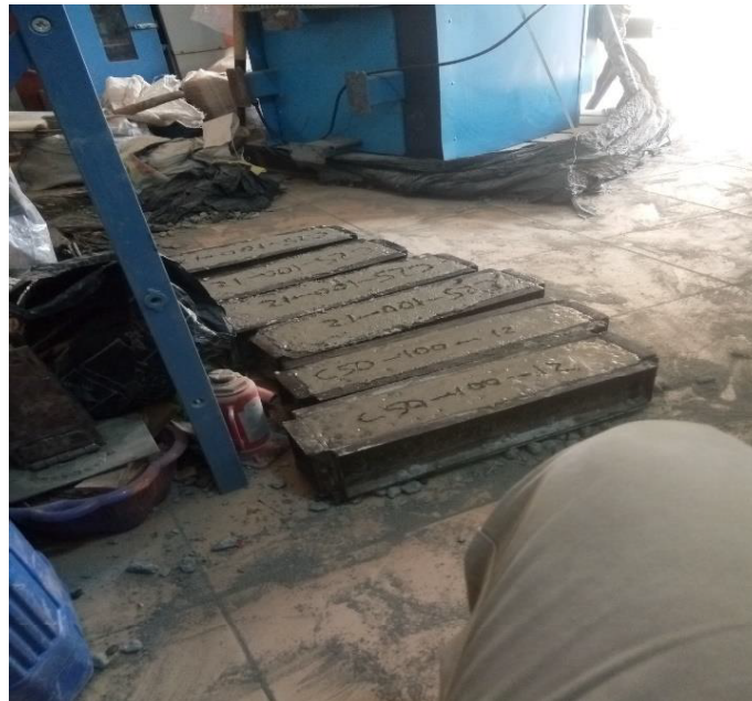
Figure 2: Concrete Beams cast with 100 X 100 X 500 Steel Moulds
