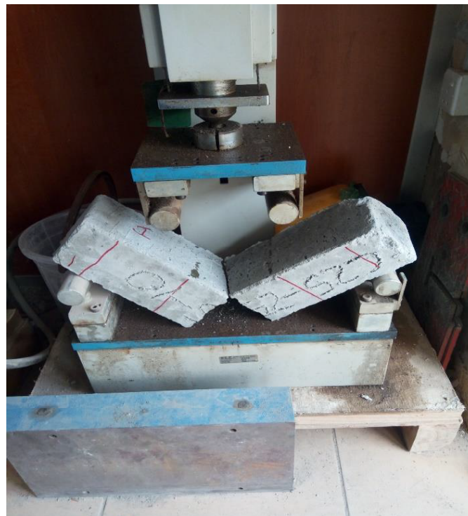
Figure 4: Beam Specimen Tested in Flexure showing Failure at the Middle Third-Span
