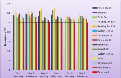
Figure 9: Temperature benchmark in comparison with the measured temperature
