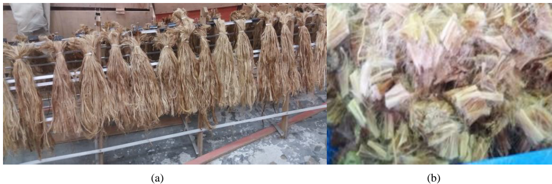
Figure 1: (a) Drying of treated Kenaf Fibre (b) Cut Kenaf Fibre ready for use
