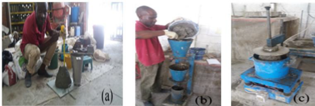
Figure 3: Measurement of (a) Slump, (b) Compacting Factor and (c) Vebe for workability test
