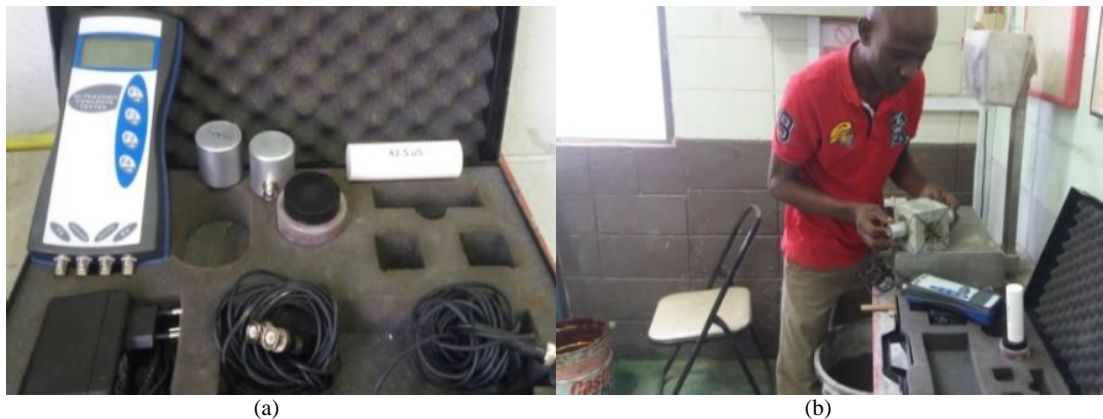
Figure 9: (a) Set-up of the UPV test (b) Operational sequence for obtaining UPV
