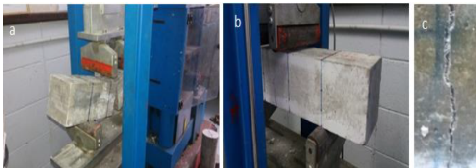
Figure 15: Failure mode of prism in Flexure (a) PC specimen (b) KBFCC specimen (c) Kenaf fibre bridge across the crack space
