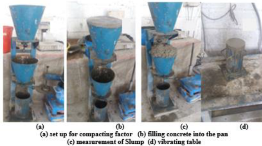
Figure 4 Operational procedures for compacting factor test
