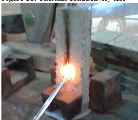
Figure 12: Fire reaction test
