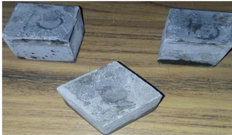
Figure 5: RPC specimens @ 27 °C
