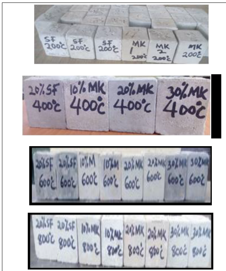
Figure 6: RPC sample exposed to elevated temperatures
