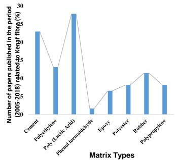
Figure 1: Percentage weight of research effort on the usage of various available matrix for Kenaf fibrous composite
