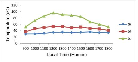
Figure 10: Daily Temperature versus Local Time for 06-02-17 on No-Load
