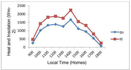
Figure 6: Heat and Insolation Profile Showing Hourly Variation for 04-02-17 on No-Load
