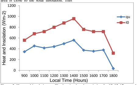
Figure 5: Heat and insolation profile showing hourly variation for 02-02-17 on no-load
