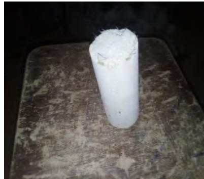
50x100mm cylinder specimen
