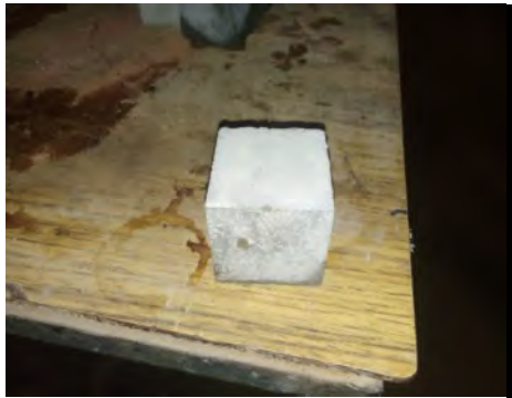
50x50x50mm cube specimen Figure 3: Concrete Specimens
