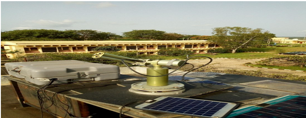
Figure 2: AERONET CIMEL Sun-photometer at block 9 of the faculty of physical science, University of Ilorin, Nigeria.
