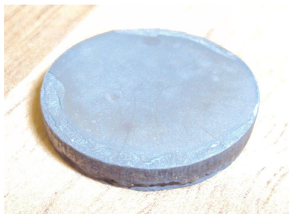
Figure 3: Macrograph of green compact from \text{TiH}_2 powder with broken corners at higher compaction pressure (>393MPa).
