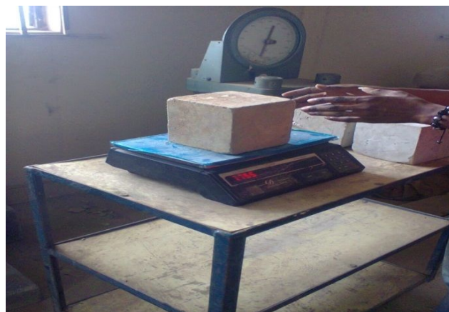
Plate 4: Weighing concrete cube
