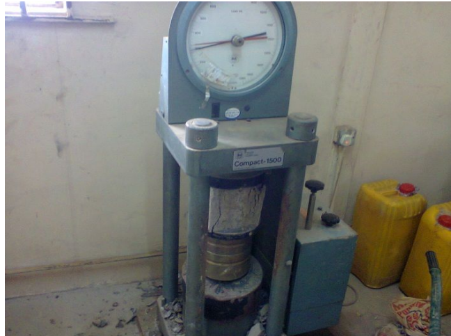
Plate 5: Crushing concrete cube on compression machine
