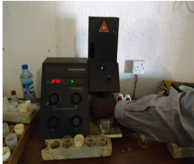
Plate 3: Flame photo spectrometer test equipment
