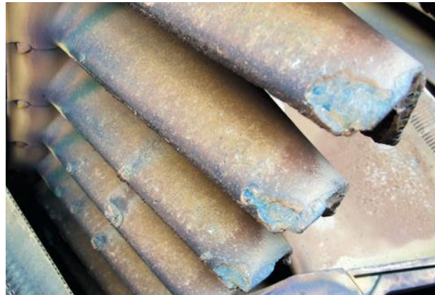
Plate 1: Degraded turbine blade tips (Bacos, 2011)
