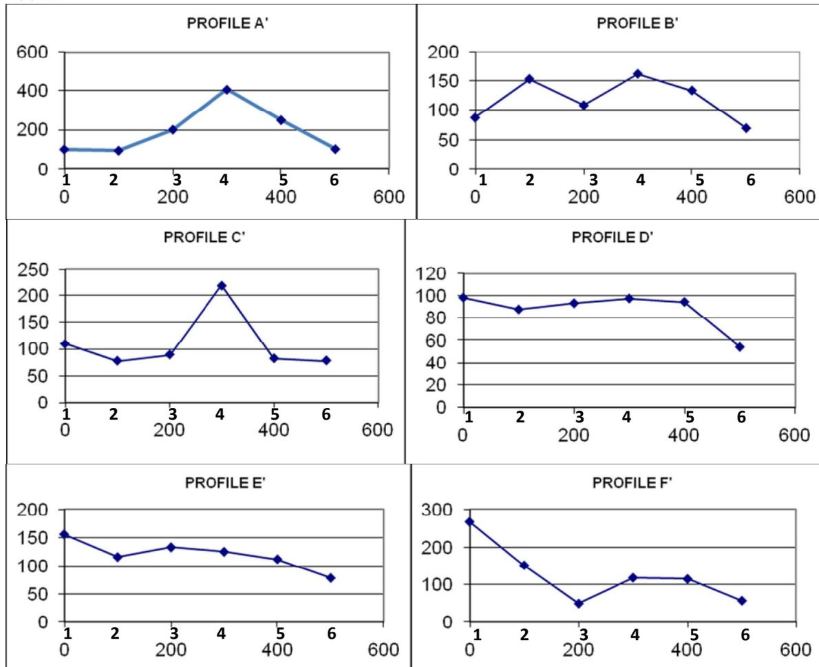
Figure 6: a - f: Wenner configuration ( $\rho$  ( $\Omega\text{m}$ ) Vs Distance (m)) for profile A' – F'
