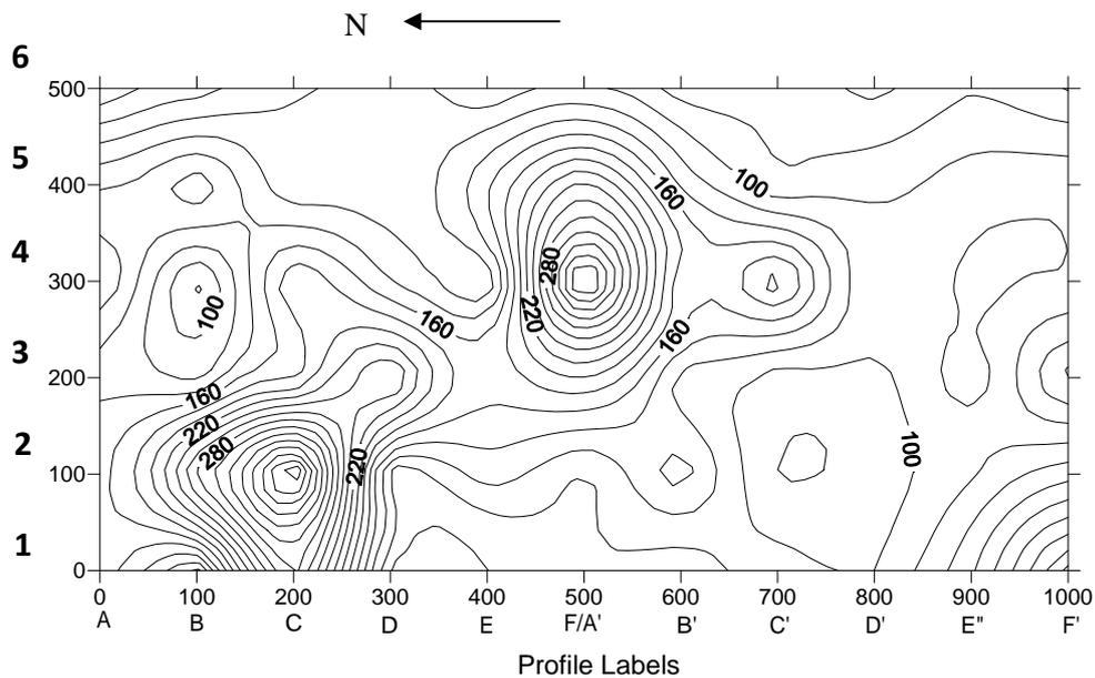
Figure 7: Contour map of Electrical Profiling at 15m Depth (Contour interval is  $20\Omega m$ )
