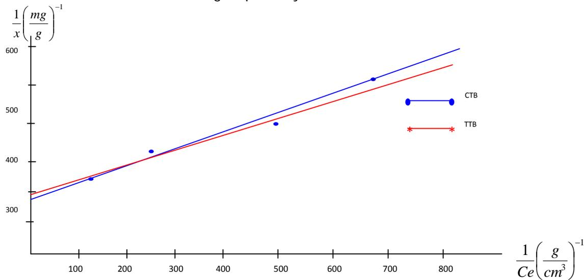
Fig. 2: A graph of 1/X vs 1/Ce using chemically and thermally treated bone based adsorbent before regeneration
