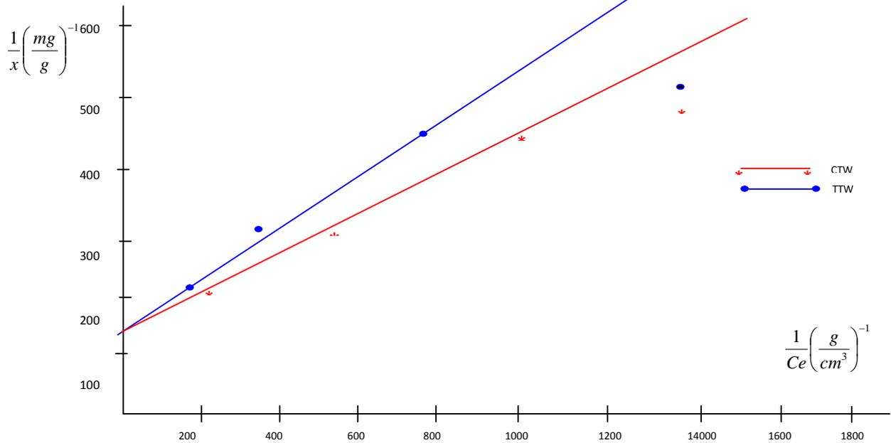
Fig. 4: A graph of 1/X vs 1/Ce using chemically and thermally treated wood based adsorbents before regeneration
