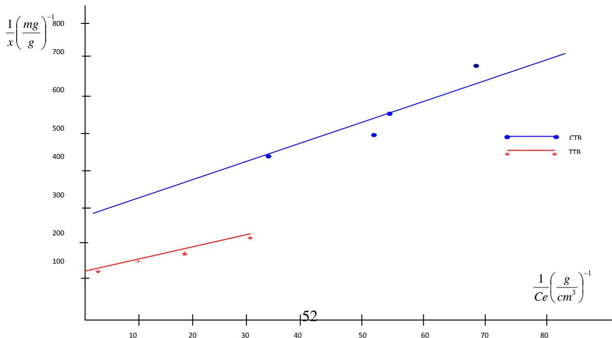
Fig. 3: A graph of  $1/X$  vs  $1/C_e$  using chemically and thermally treated bone based adsorbent after regeneration
