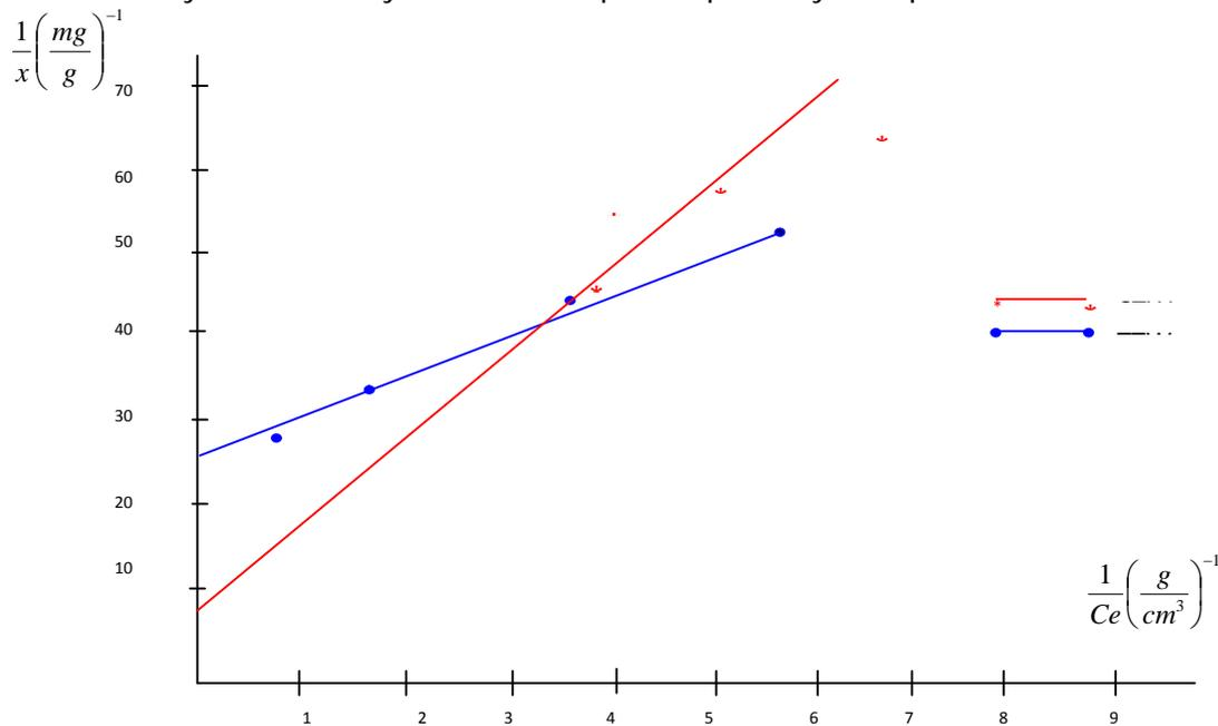
Fig. 5.0: A graph of 1/X vs 1/Ce using chemically and thermally treated wood based adsorbents after regeneration
