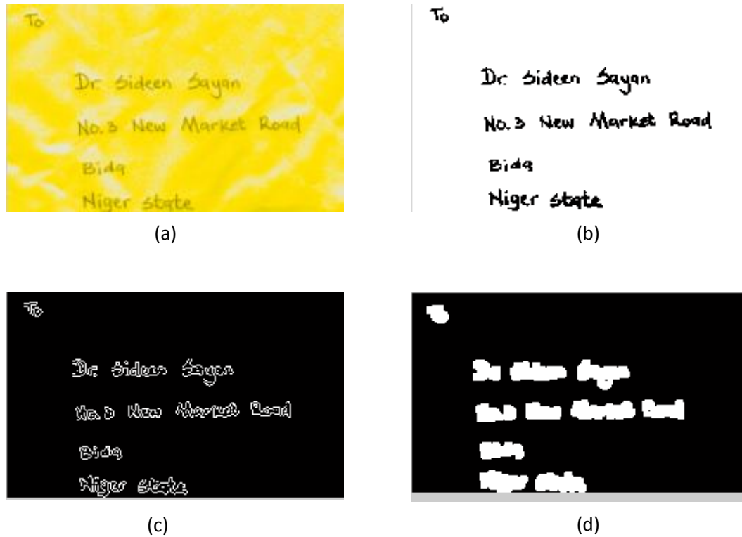
Figure 6: Intermediate stages of processing (a) original address envelop; (b) image segmentation; (c) after edge finding; (d) after binarization and dilation.
