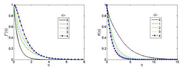
Figure 5: Effect of Gr on the velocity and temperature profiles
