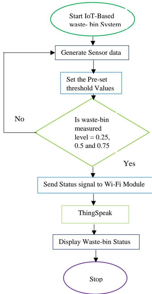
**Figure 3: Flow Chart of the Implemented System**
