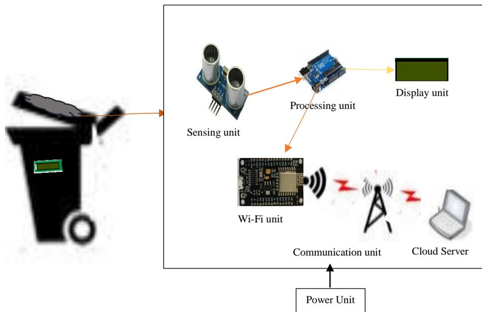
**Figure 1: The Schematic Diagram of an IoT-based Waste Monitoring System**
