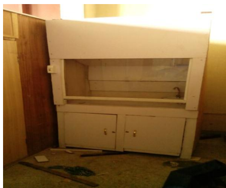
Plate 3: The fabricated Fume cupboard
