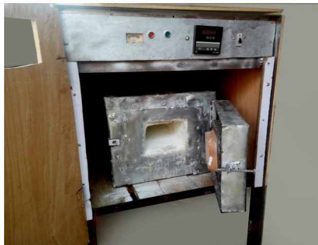
Plate 6: Pictorial inside view of the developed muffle furnace
