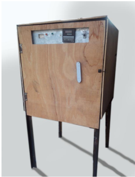
Plate 4: External casing of the muffle furnace
