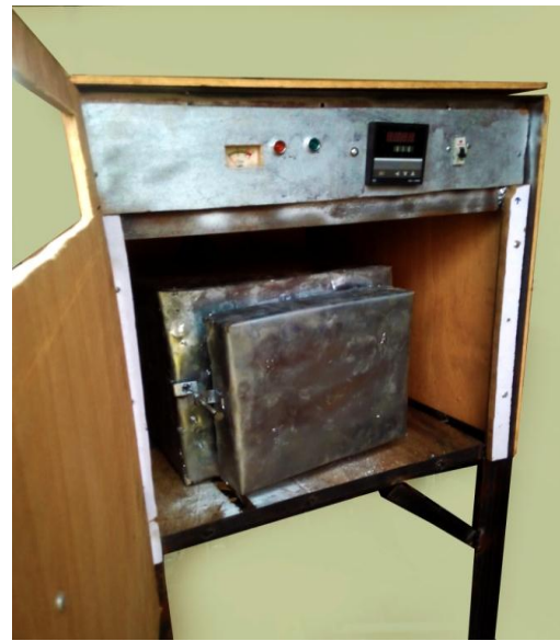
Plate 5: Front view of the developed muffle furnace
