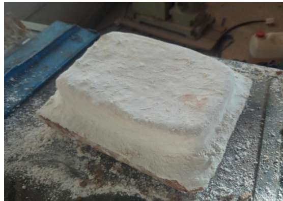
Plate 2: Moulded furnace door
