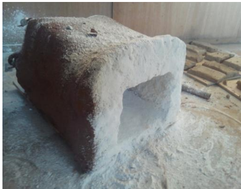
Plate 1: Moulded heating chamber
