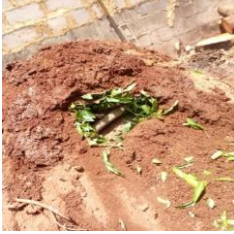
Fig. 3: Conventional Carbonization Chamber
