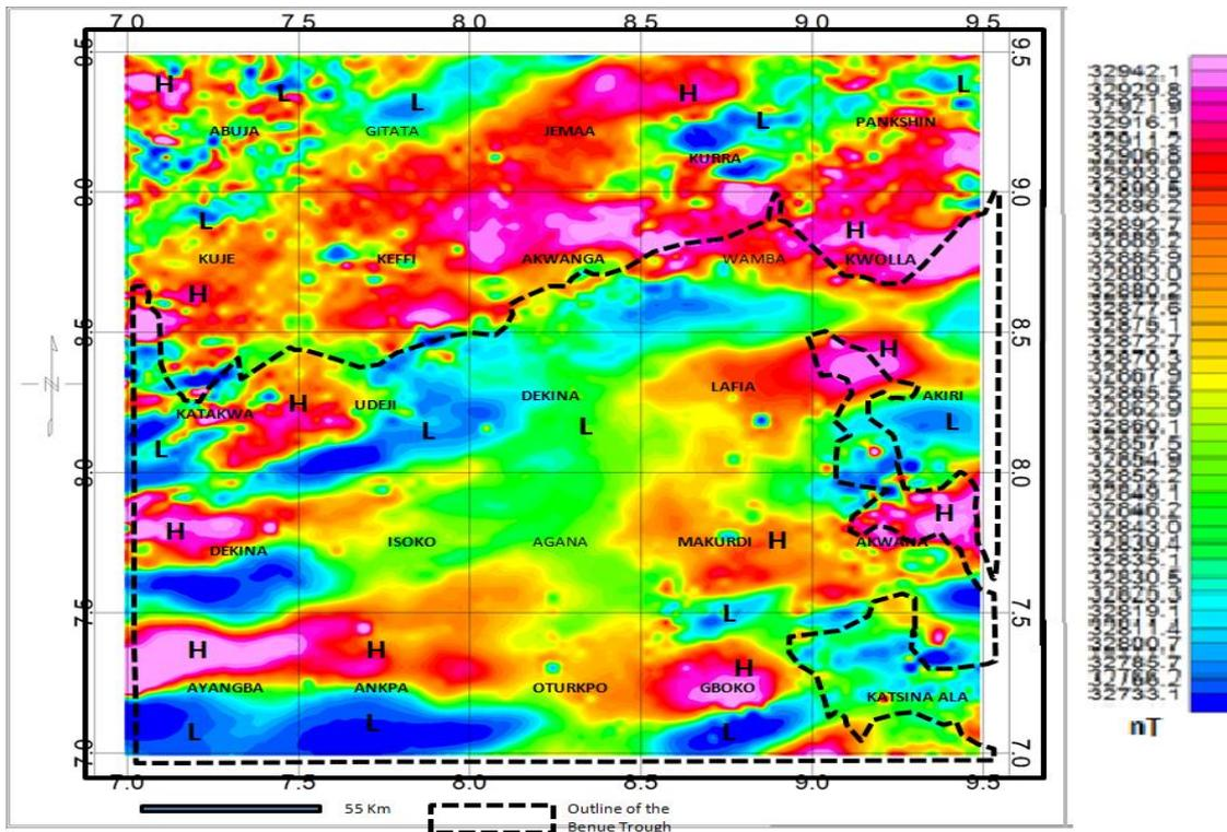
**Figure 2: Total Magnetic Field Intensity Map of the Study Area showing areas of Magnetic Highs and Lows**
