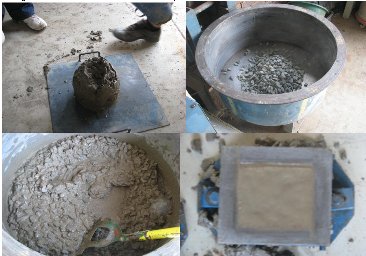
Figure 1 Batching, Mixing and cast concrete
