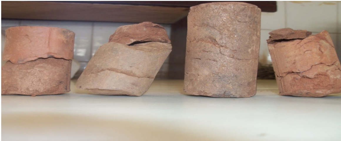
Plate III: Cracked Clay Rods
